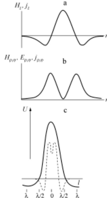
**Fig. 2.** Radial dependence of components of the vectors  $\mathbf{E}$ ,  $\mathbf{H}$ ,  $\mathbf{j}$  for the principal radially symmetric mode (a, b); dependences of the voltage  $U$  proportional to the component  $H_z$  on the distance  $l$  expressed in half-waves (c).
