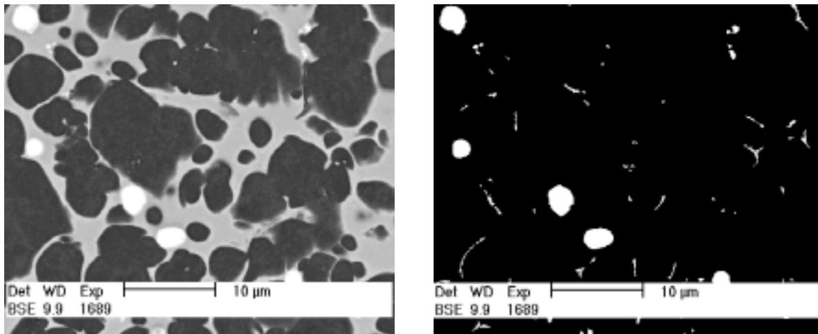
**Figure 3.** The sintering phase before (left), and after the image processing (right). White areas are holes.
