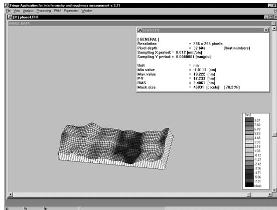
Fig. 6. Three – dimensional map the surface of gauge block.
