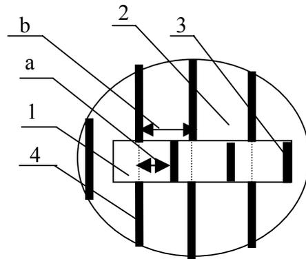
Fig. 2. 1 – gauge block, 2 – reference plate, 3 – fringe on the surface of gauge block , 4 – fringe on the surface of reference plate, a – length, which corresponds to the fringe fraction  $u$ , b – length between two fringes on the reference plate.
