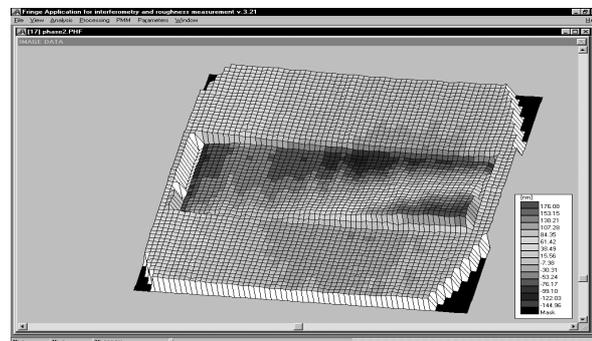
Fig. 5. Three – dimensional map the surface of gauge block and reference plate.
