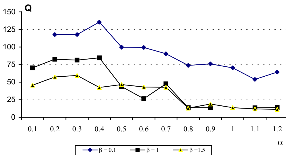
Fig. 3. Correction effectiveness index Q in function \alpha for three values \beta for the first-order inertial measurement channel.
