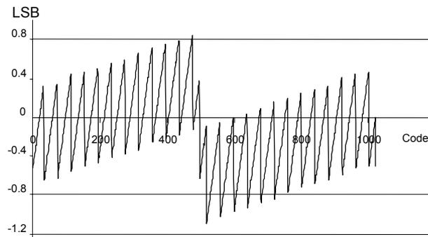
Fig.9. INL Results from VHDL-based test
