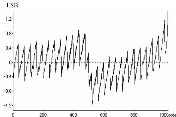
*Fig. 11. INL Results from dynamic test equipment*
