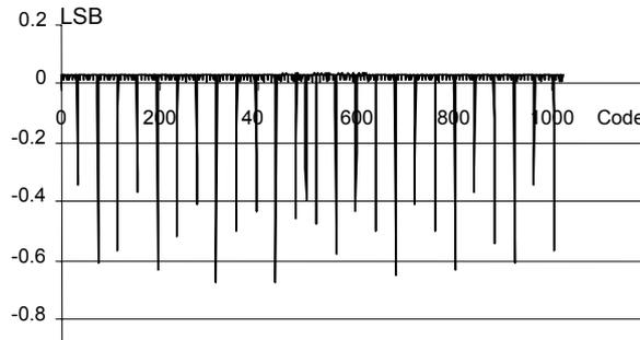
Fig.8. DNL Results from VHDL-based test
