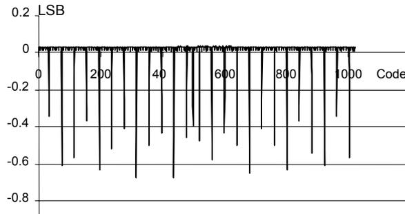
Fig.8. DNL Results from VHDL-based test
