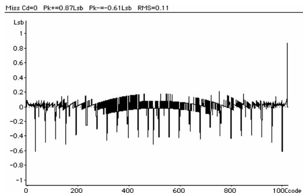
Fig. 10. DNL Results from dynamic test equipment
