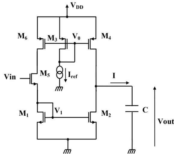
Fig. 2. Elementary cell of the CCO
