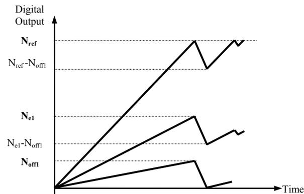
Fig. 5. Count-discount procedures of the  $U_{DC}$
