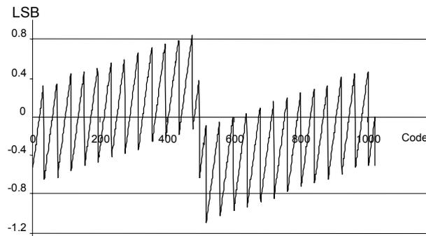
Fig.9. INL Results from VHDL-based test
