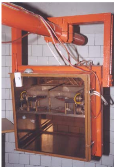
Fig. 1 A cabin of the centrifuge for testing of 2 experimental animals (rats). Each animal is connected to four syringes driven by two stepping motor. 10 cabins are placed on the centrifuge arms with a length of 3 meters.
