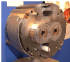
Fig. 3. Cross section of the magnet
