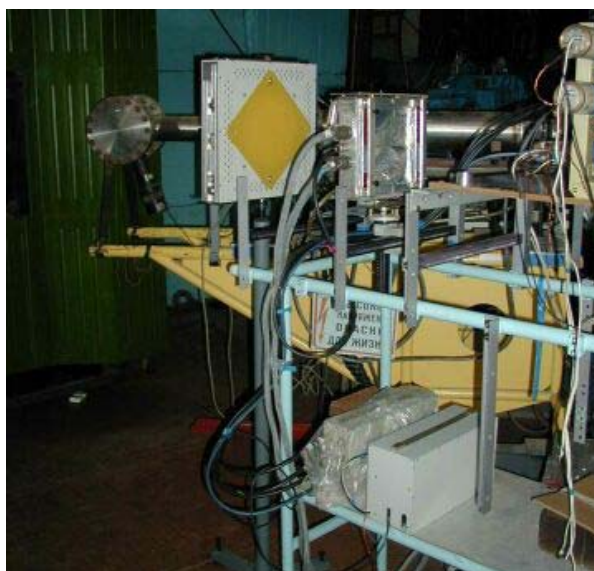
Fig. 2. Apparatus for the beams spatial parameters measurement
