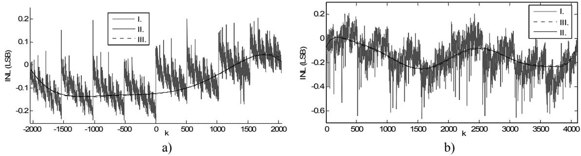
Fig. 1. Measured and modelled  $INL(k)$  for 12b ADCs a) Lab-PC-1200, 5 harmonic components used b) ADuC812, 9 harmonic components used I.)  $INL(k)$  measured by histogram method 1MS record II.) First method (recurrent best fitting) 100kS, 97.1Hz III.) Second method (spline interpolation, coherent resampling and FFT) 65.5kS, 43.2Hz
