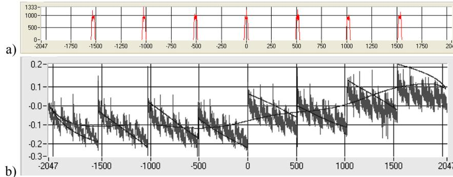
Fig. 2.  $INL$  of LAB-PC-1200 data acquisition card modelled by two component model. The  ${}^{LCF}INL_m(k)$  obtained by spectrum analysis and  ${}^{HCF}INL_m(k)$  determined by reduced amplitude triangular histogram test. a) histogram b) measured and modelled  $INL$ .
