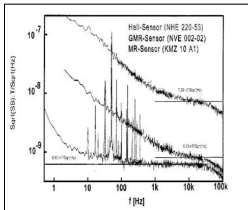
Fig. 1 – Noise spectra of Philips KMZ10A1, GMR sensor NVE AA002-02 and Hall sensor NHE 220-53
