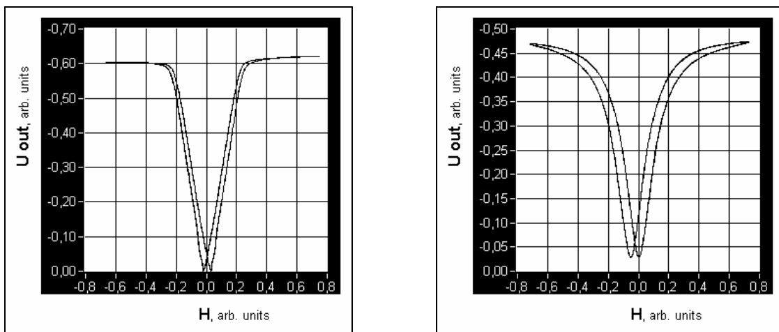
Fig. 3 – Sensor characteristics example of two commercially available GMR sensors
