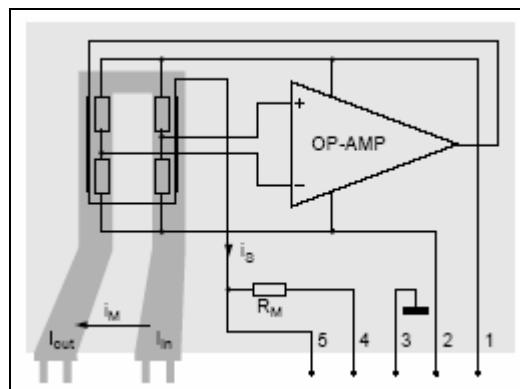
Fig. 2 – The functional scheme of the module Sensitec CMS2000 [6]
