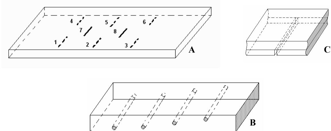
Fig. 4 – Test situation: A – aluminium test plate with slots (220x120x5 mm, slots 1÷6 on bottom, slots 7 and 8 on top; depth of the slots: 1: 3 mm; 2: 2 mm; 3: 1 mm; 4: 0,8 mm, 5: 0,6 mm; 6: 0,4 mm; 7: 0,8 mm; 8: 0,6 mm; conductivity of the alloy is 19 MS/m), B – aluminium block 410×100×25 mm with through holes Ø3 mm on depth 2,5 / 5 / 7,5 / 10 mm, C – border line between two aluminium plates through aluminium plates of various thickness placed on top
