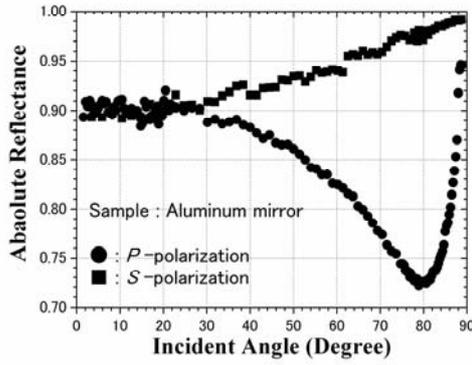
Fig. 4 Absolute reflectance of an aluminum mirror.
