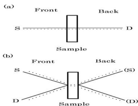
Fig.1 Symmetry X system for optical measurement. S is a light source and D is a detector.
