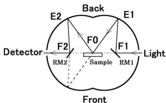
Fig. 2 Block diagram of STAR GEM
