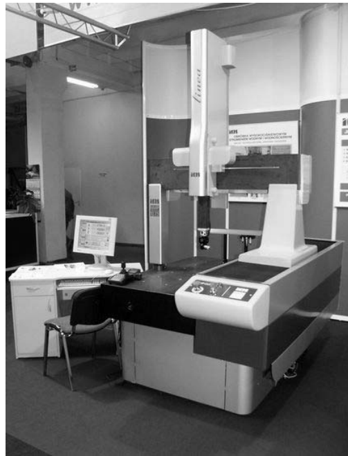
Fig. 2. NMP Linea MP_E = 3.5 \pm 1/250 \mu\text{m} .
