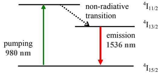
Fig. 1. The three-level system of optical pumping in the Er<sup>3+</sup> ion.
