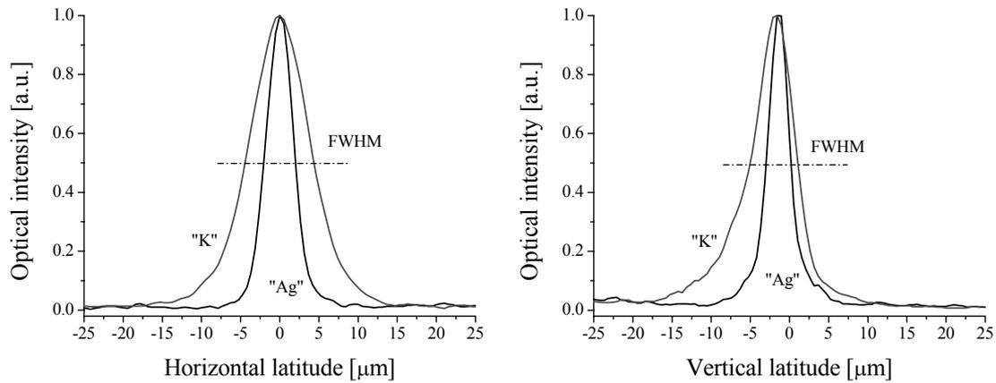
Fig. 2. Horizontal (on the left) and vertical (on the right) cross-section of the mode intensity profile of the single mode glass channel waveguides at 1500 nm. The waveguides fabricated by Ag<sup>+</sup> ↔ Na<sup>+</sup> and K<sup>+</sup> ↔ Na<sup>+</sup> ion-exchanges are compared (same width of the mask).
