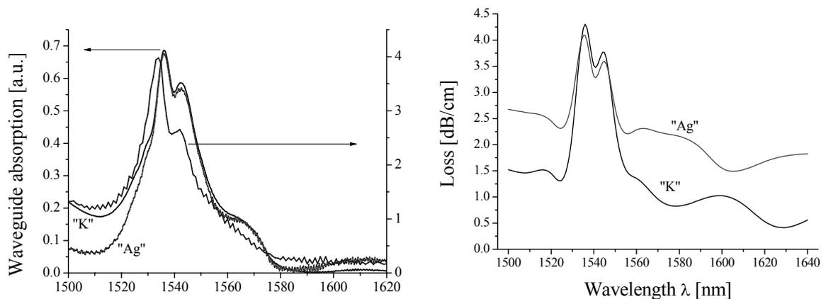
Fig. 3. Absorption spectral dependency of the glass substrate, “K” and “Ag” channel waveguides - on the left. Spectral dependency of optical loss in channel waveguides (same width of the mask) - on the right.
