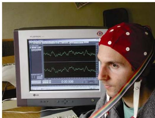
Fig.2.: EEG montage realized by EEG cap with electrodes placed according to International 10-20 system.
