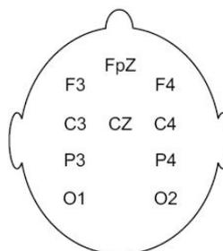
Fig.3.: Placement of active electrodes. Reference and ground electrodes placed at Cz and Fpz points, respectively.
