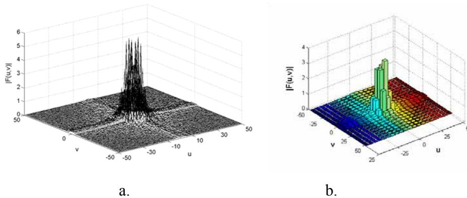
Fig. 2. a/ Frequency spectrum, b/ modified frequency spectrum of corrected image of visualized polymeric foil OOL30
