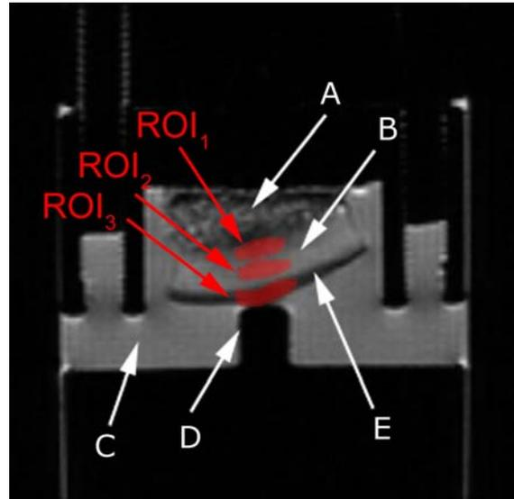
Fig. 1. Cartilage specimen in micro-imaging system (SE sequence used, TR = 4s, TE = 15ms): A – bone tissue, B – deep zone of cartilage (radial zone), C – PBS + GdDTPA<sub>2</sub>- solution, D – compressive part of piston, E – superficial zone of cartilage (transitional zone), ROIs defined for different cartilage zones (1 - deep, 2 - radial, 3 - superficial).
