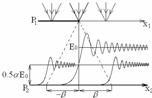
Fig. 3. Edge Fresnel image under non-uniform harmonic type illumination.
