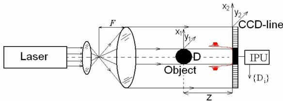
Fig. 1. Structure scheme of the Fresnel meter.
