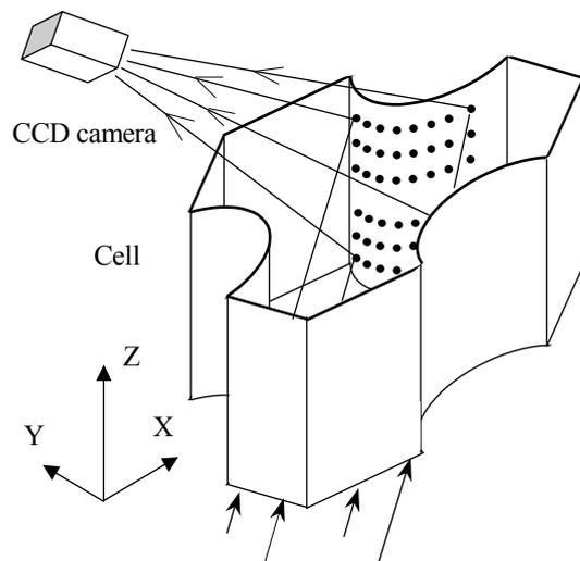
Fig. 14. The multipoint structured illumination 3D inspection method applied to a single segment of grid spacer cell.
