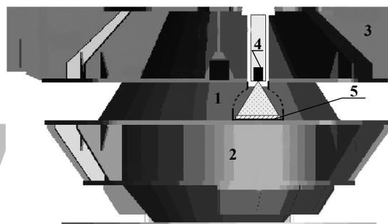
Fig. 8. Measurement system location on oil-drilling platform: 1 - slider bearing, 2 - support, 3 - platform, 4 - image unit, 5 - target.
