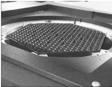
Fig. 12. A grid spacer for reactor VVER-1000.
