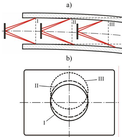
Fig. 6. Modification of the ring mark image versus the hole axis bending; a – object with axis bending; b - ring mark image.
