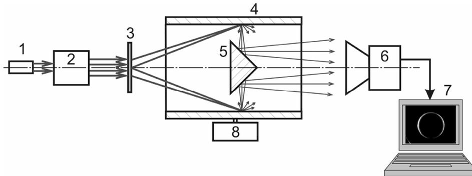
Fig. 5. Principle of holes inspection by DOE: 1 – laser; 2 – collimator; 3 – DOE; 4 – object under inspection; 5 – conical mirror; 6 – CCD-camera; 7 – computer; 8 – device for detail moving.
