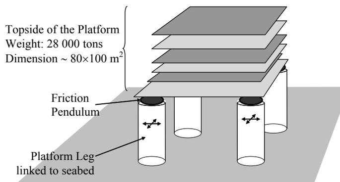
Fig. 7. An oil-drilling platform scheme.
