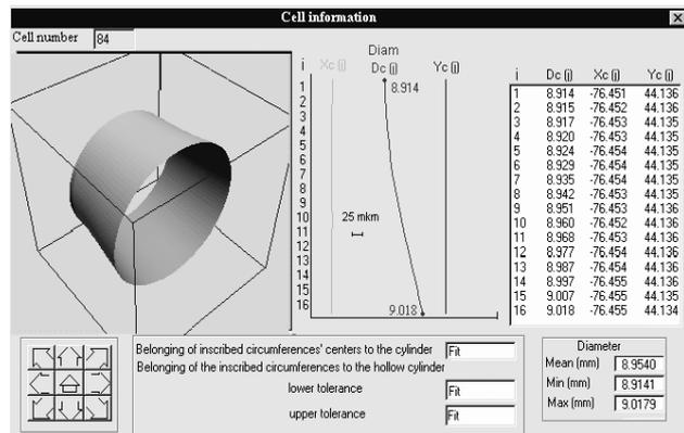
Fig. 16. The individual geometric information from LMM about every cell hole of the grid spacer: its 3D image, the diameters  $D_c(j)$  and the centers coordinates  $X_c(j)$ ,  $Y_c(j)$ .
