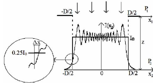
Fig. 2. Slit Fresnel image.  $P_1$  and  $P_2$  are object and image planes.
