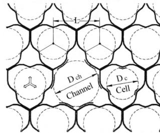
Fig. 13. The grid spacer geometric parameters under inspection.
