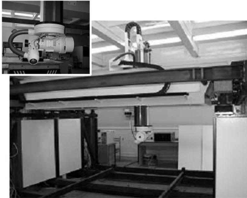
Fig. 11. Laser technological system LSP-2000 and enlarged fragment of its working processing head.
