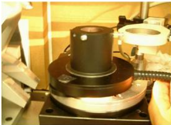
Fig. 6. Special ring-light adapter to create dark-field illumination. Left: photograph of the adapter; right: direction of light rays [3].
