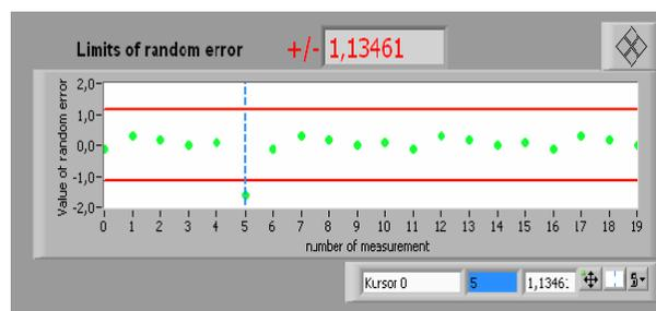
Fig.1 Panel of virtual device designed to verify gross errors
