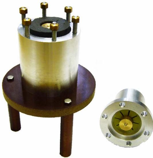
Fig.4 Physical realisation of the coaxial flange
