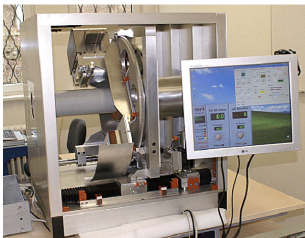
Fig. 12 Photo of developed X-CT equipment including the main control computer with touch-screen LCD panel.
