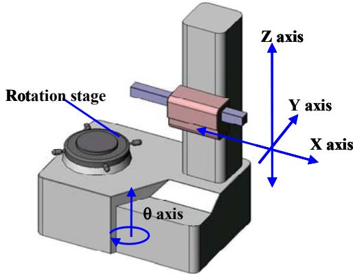
Fig.2 Measurement system of scroll profile
