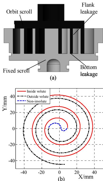
Fig.1 Leakages of scroll compressor and measurement profile
