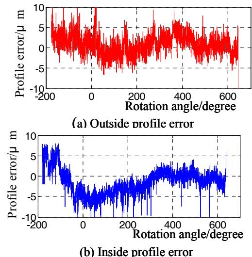
Fig.5 Measurement result after error separation
