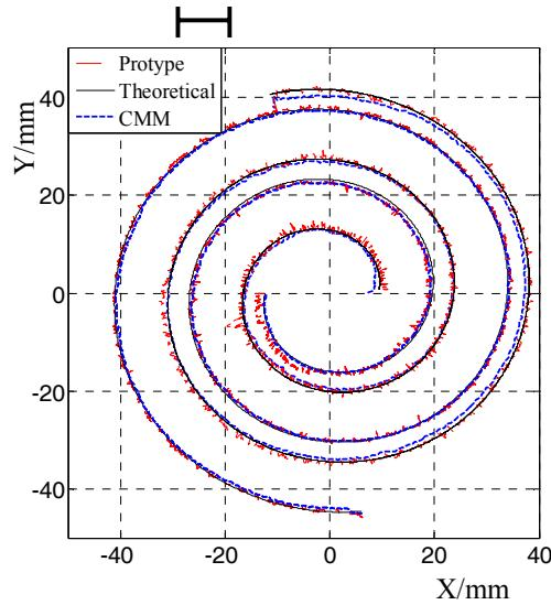
Fig.6 Measurement results for involutes profile of scroll
