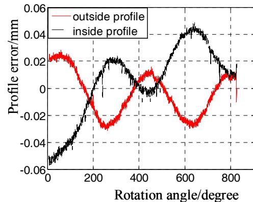
Fig.3 Measurement result without error separation
