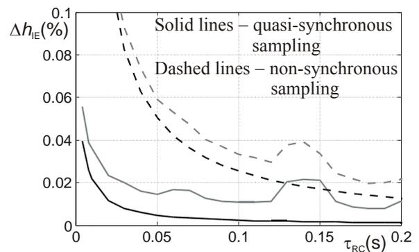
Fig. 3. Error of IE in the middle of range (theory – black, simulation – gray).
