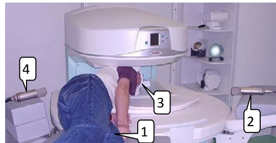
Fig.7. A speech and noise recording experiment arrangement: bed with testing person (1), front read microphone 1 (2), patient's head in RF coil (3), back read microphone 2 (4).
