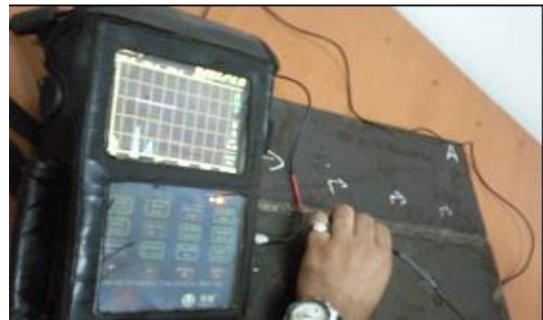
Fig.3. Measurement set-up: the ultrasound device and a welded steel sample.
