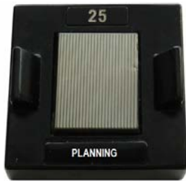
Fig.4. Machined surface produced by planning V9.
