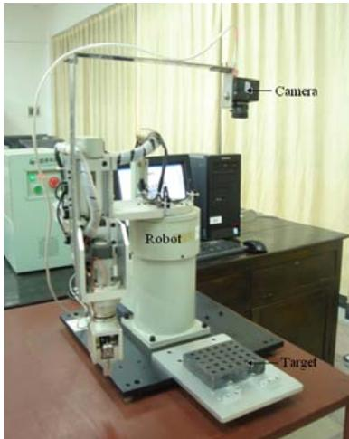
Fig.5. Vision system and manipulator
