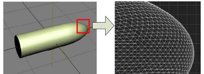
Fig.3. the 3D digital model of the projectile with its triangular mesh surface.
