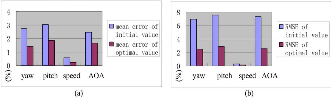
Fig.7. Comparison between the initial and optimal values: (a) the mean values of the relative errors; (b) RMSE of the relative errors.
