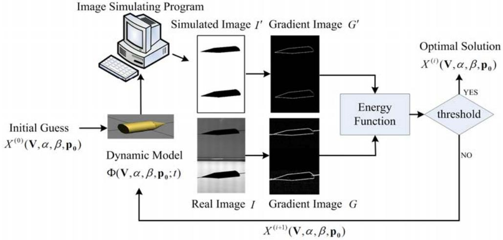
Fig.4. The flow of motion parameter estimation.
