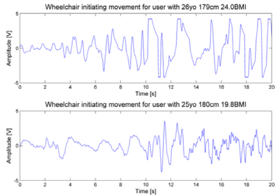
Fig.10. Twenty seconds of backrest ICG using the copper board displayed in Fig.5. embedded within the wheelchair backrest as sensing module, obtained for two subjects when the wheelchair initiates motion. When motion starts, baseline oscillations dominate the ICG. One subject (top) displayed a regular ICG for the first seconds, but it was obliterated during movement and the other (bottom) although avoiding saturation did not produce a visible ICG during motion.
