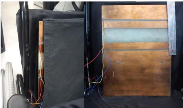
Fig.5. Photographs of the ICG transduction board with a large reference electrode and close sensing electrodes. Built from a single-sided printed circuit board with FR4 substrate (right), and partially embedded in a cover placed over the wheelchair's backrest (left). A ruler with a 20 cm range is shown for scale.
