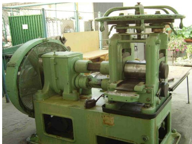
Fig.2. Two-high rolling stand DUO 210 SVa.
