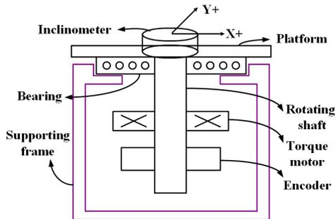
Fig.1. Rotating shaft tilt angle measurement mechanical structure.
