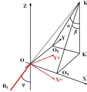
Fig. 7. Projection of rotating shaft tilt angle.
