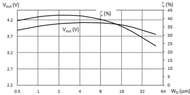
Fig.8. Option 2: Efficiency and output voltage as functions of  $W_D$ .
