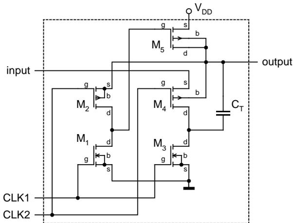
Fig.1. One cell of the proposed charge pump [8].
