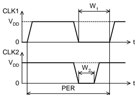
Fig.2. Waveforms of 2-phase clocks.
