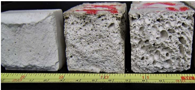
Fig.7. Structure of the materials with different bulk density. From left: reference material G (bulk density 964 \pm 20 \text{ kg/m}^3 ), GL14 ( 736 \pm 18 \text{ kg/m}^3 ), GL17 ( 586 \pm 19 \text{ kg/m}^3 ).
