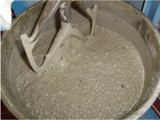
Fig. 2. Preparation of the foamed material in the laboratory mixer.
