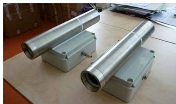
Fig.8. Two AK-UTEE-v2 measuring systems for measuring negative and positive ions.
