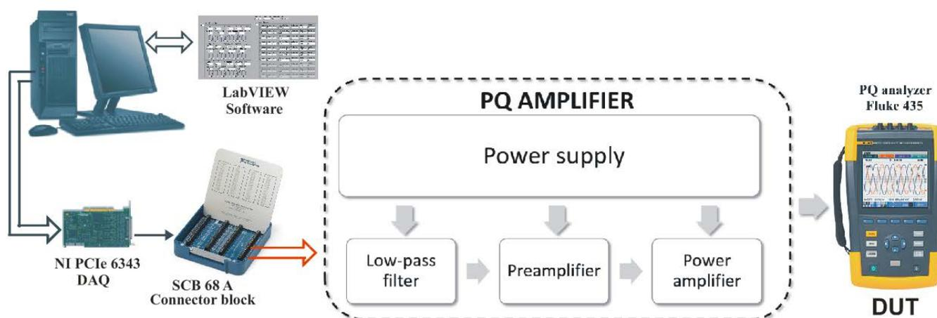
Fig.5. Block diagram of experimental procedure for testing quality analyzer Fluke 435 using LabVIEW based signal generator.
