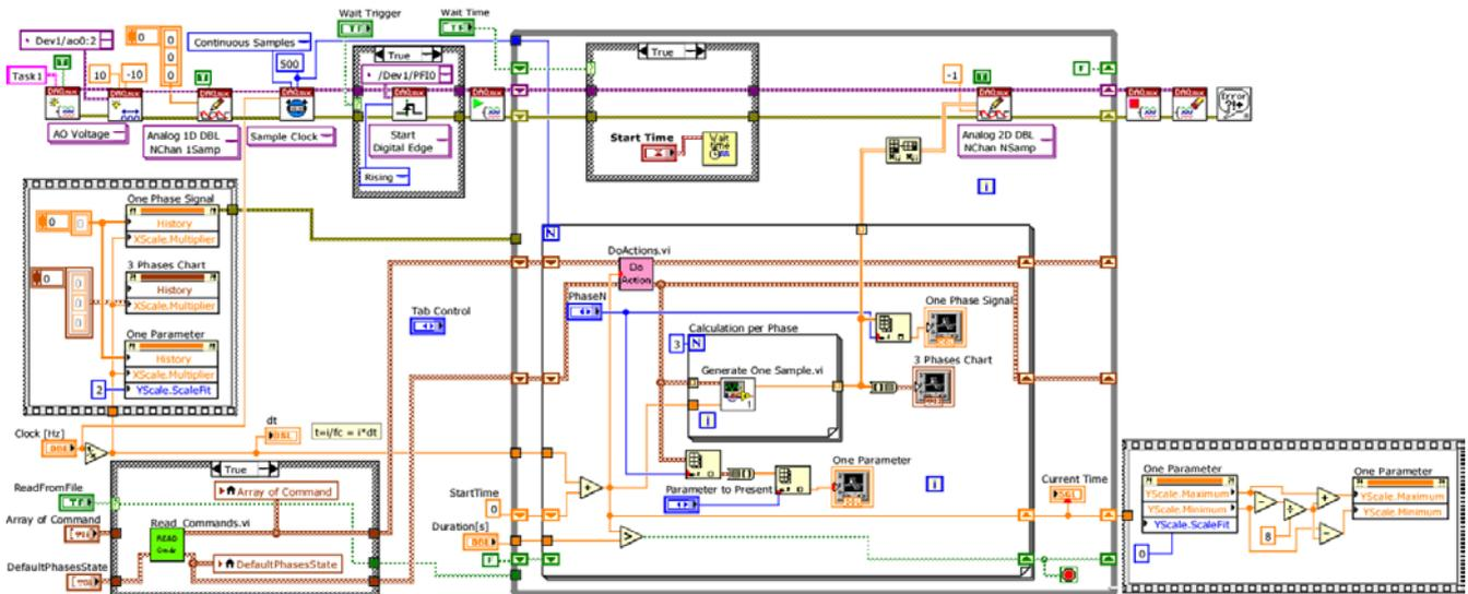
Fig.4. Block diagram (software code) of LabVIEW virtual instrument for generation of VQ signal disturbances.
