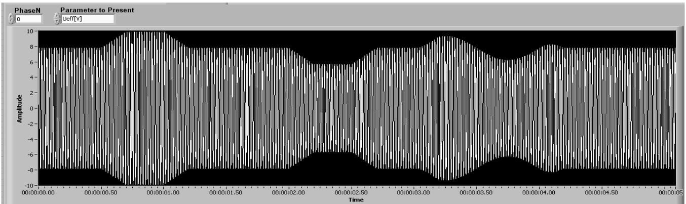
Fig.2. Graphical presentation of voltage test signal with various disturbances generated using LabVIEW based virtual instrument.
