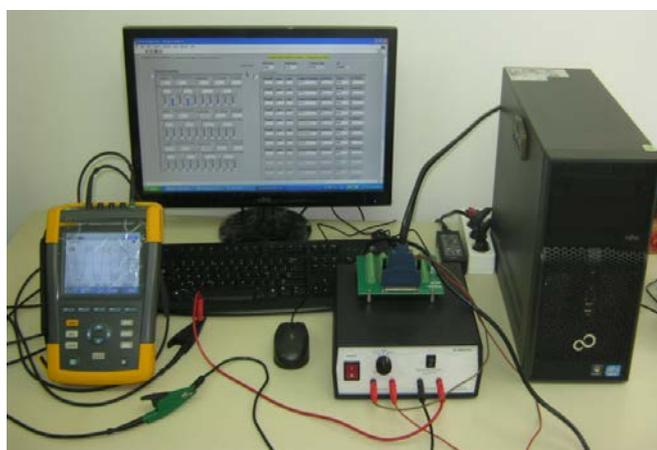
Fig.6. Photo of experimental system for testing instrument Fluke 435 using LabVIEW based signal generator.
