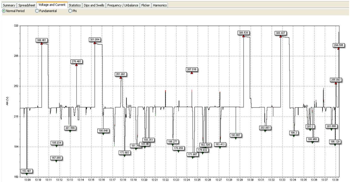
Fig.8. Time diagram of measured RMS voltage values - 30 minutes long test signal with large number of voltage disturbances.
