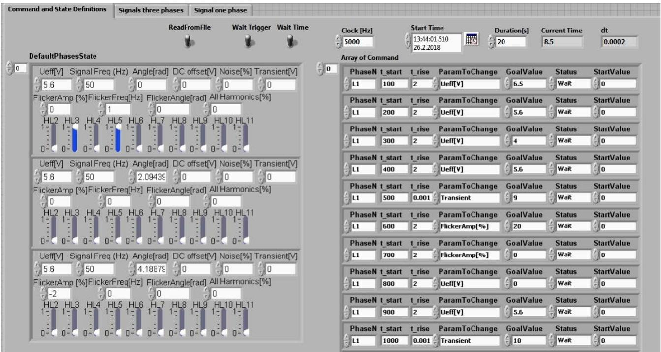
Fig.1. Control front panel of LabVIEW virtual instrument for generation of standard VQ signal disturbances.
