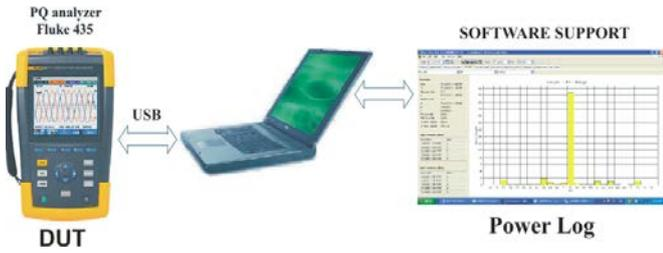
Fig.7. USB communication between instrument Fluke 435 and computer for recording and processing of measurement data.
