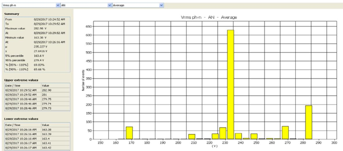
Fig.11. Time diagram (above) and histogram (below) - measured RMS voltage values (300 s long test signal, no harmonics, flicker 10 %).
