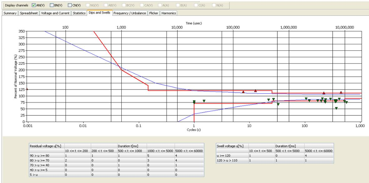
Fig.10. Power Log software analysis of detected signal disturbances according to the quality standard
