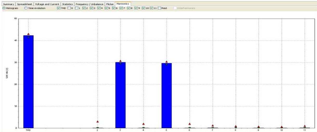
Fig.12. Histogram of measured high-order signal harmonics (total THD value, 30 % of H3 and H5 voltage harmonics).
