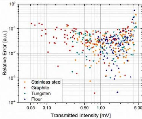
Fig.6. Relative error in function of transmitted intensity. The experimental data confirm the numerical model. We have an asymptote for the transmitted intensity which goes to  $I_w$  and to zero.
