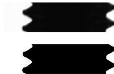
Fig.9. Thread image of extremum position and thread image after pre-processing.
