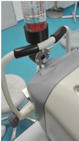
Fig.2. Developed standard's eye model with the artificial cornea used during non-contact eye tonometer measurements.
