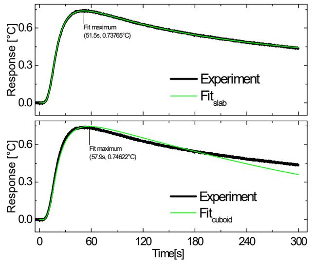
Fig.3. Fitted curve of Temperature response for time window 0-300 seconds using the slab model (top) compared with the cuboid model (bottom) for 10 s pulse width.
