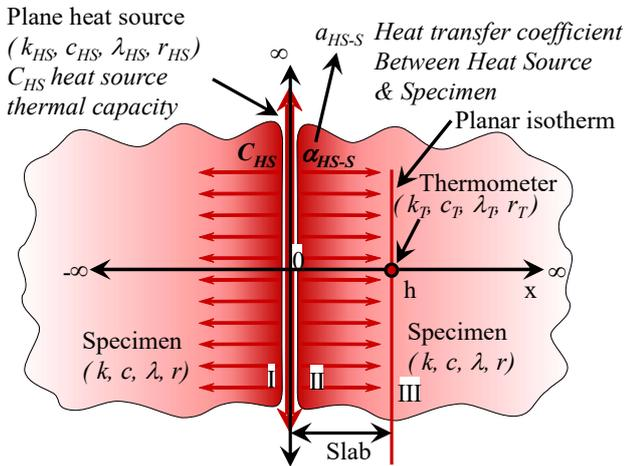
Fig.2. The slab model for infinitely large specimens accounting the heat source heat capacity as well as the heat transfer coefficient in between the heat source and specimen body is drawn with the experimental parameters and geometry of arrangement [15], [16], [17], [18], [19].
