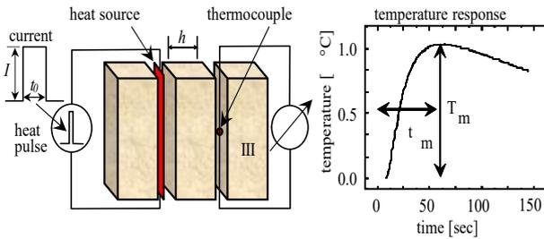
Fig.1. Principle of Pulse Transient Technique and the example of the maximum of thermal response ( $T_m$ ) is recorded in time ( $t_m$ ) to the heat pulse on the right [15], [16], [17], [18], [19].
