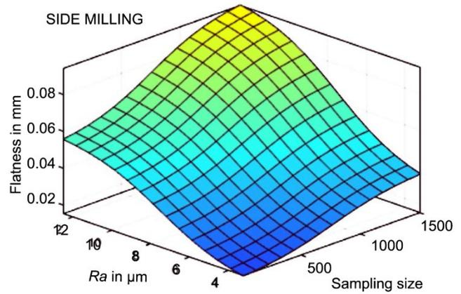
Fig.11. Influence of sampling size and surface roughness on flatness in side milling operation.
