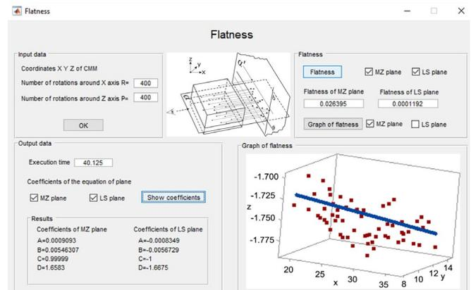
Fig. 2. Flatness error assessment using the MZ method in non-commercial software.
