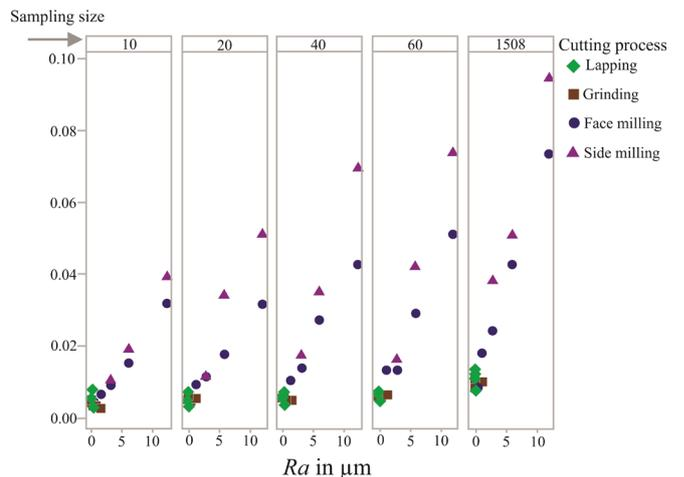
Fig.6. The effect of roughness and type of the cutting process on flatness error with different numbers of points.
