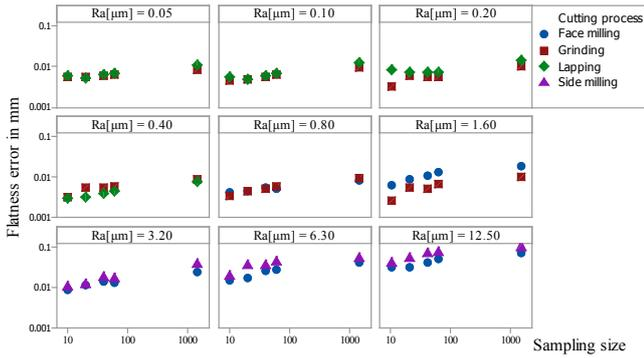
Fig.4. The effect of the number of points in the measurement strategy, surface roughness and the applied cutting process on flatness error measured on a CMM.
