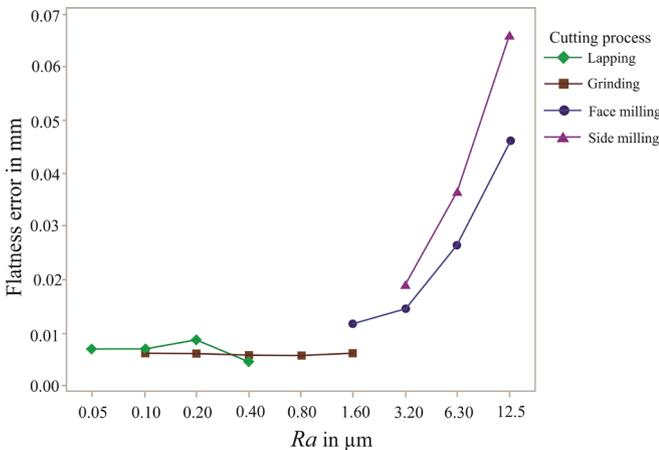
Fig.5. The effect of the cutting process and quality of the machined surface on flatness error.
