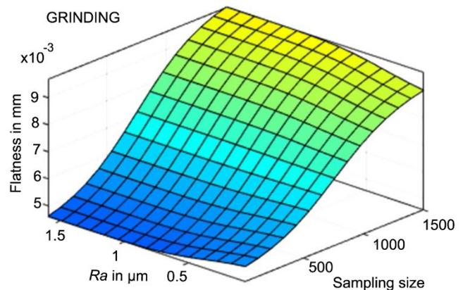
Fig.13. Influence of surface roughness and sampling size on flatness in grinding operation.
