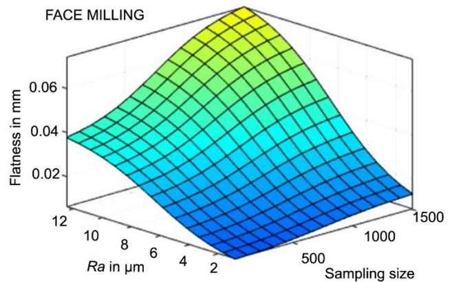
Fig.12. Influence of sampling size and surface roughness on flatness in face milling operation.
