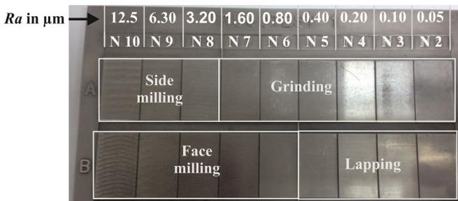
Fig. 1. Rugotest used in the experiment.
