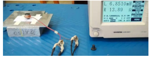
Fig. 5. Experimental setup of T-core coil above the layered conductor with a surface hole.
