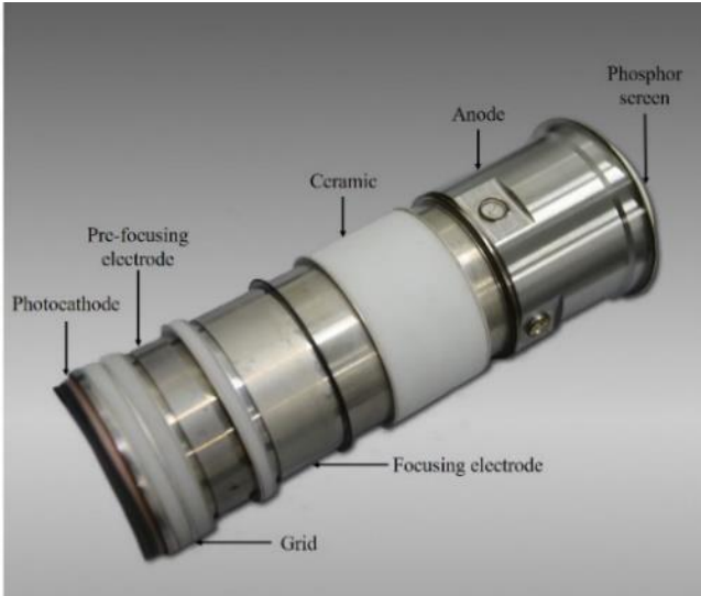
Fig. 4. A miniaturized streak tube with high luminance gain.
