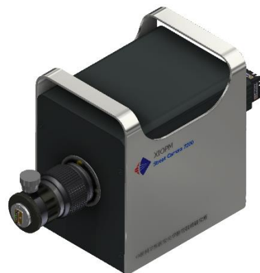
Fig. 3. A miniaturized streak camera.
