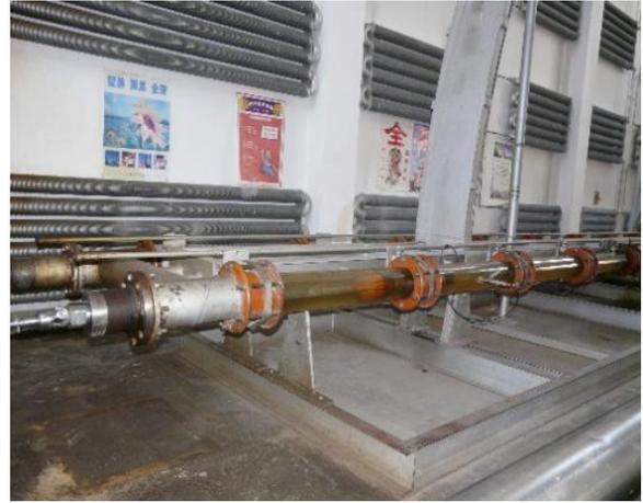
Fig. 24. The new capacitive logging instrument.
