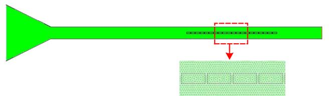
Fig. 6. Two-dimensional simulation model of the annular measurement area of the new tri-electrode capacitive sensor.
