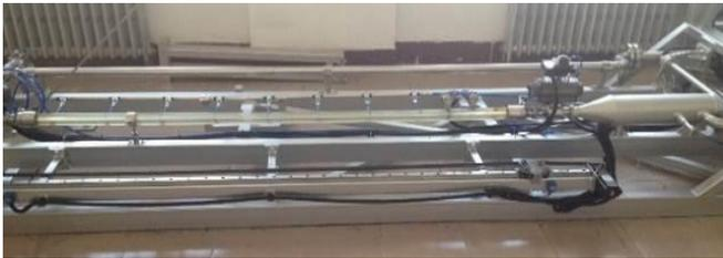
Fig. 7. A DN20 simulator for measuring the pipeline of the capacitive sensor.
