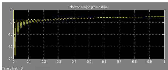
Fig. 2. Metrological transients of the initial CCVIT design project current error
