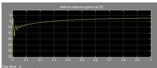
Fig. 1. Metrological transients of the initial CCVIT design project voltage error
