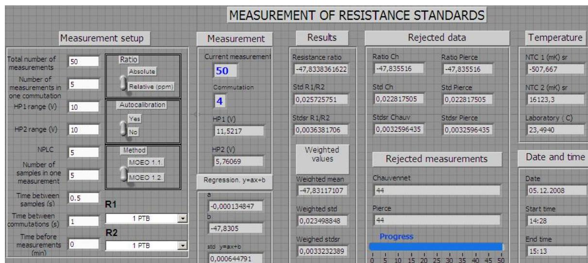
Fig. 5. Labview front panel for the measurement of resistance standards
