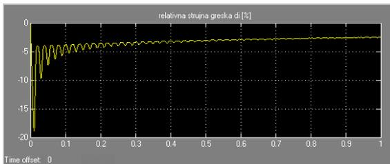
Fig. 4. Metrological transients of the optimal CCVIT design project current error
