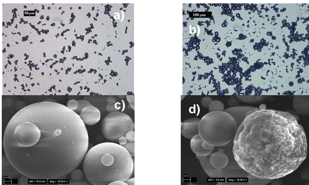
Fig. 1 Optical micrographs of the microspheres A60 (a) and A75 (b), and the detailed SEM micrographs of the same specimens, A60 (c) and A75 (d).
