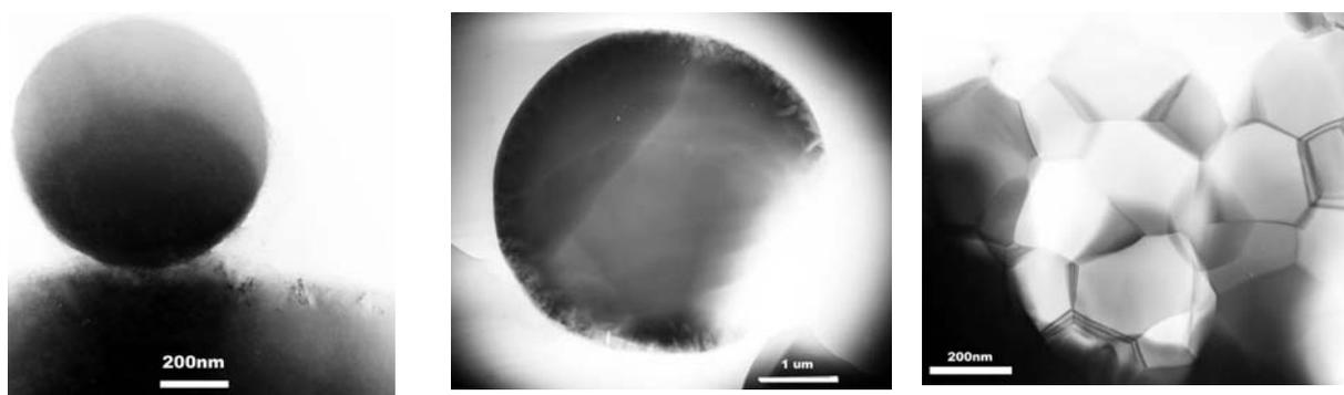
Fig. 3 TEM micrographs of prepared glass microspheres: a), A43, small, completely amorphous microsphere, b), A75, larger microsphere with surface crystallization, c) A57, polycrystalline microsphere with microstructure resembling polycrystalline  $\alpha$ -Al<sub>2</sub>O<sub>3</sub> or YAG.
