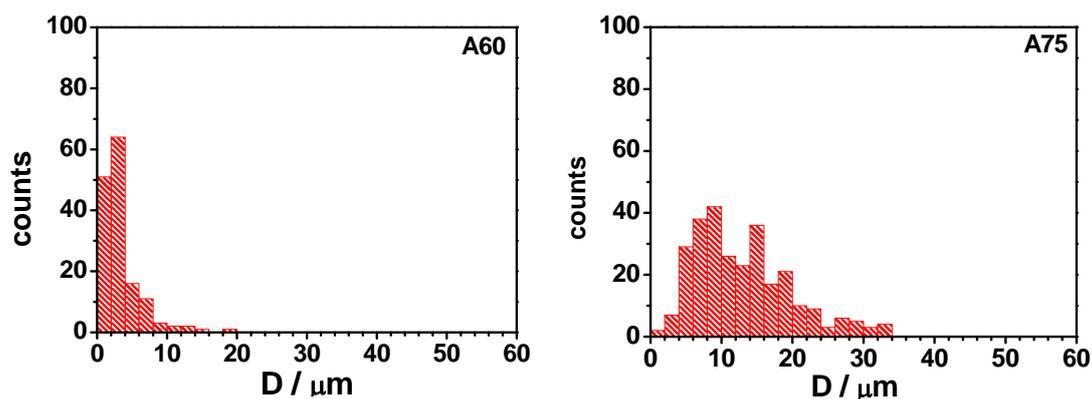
Fig. 2 Distribution of diameters of microspheres of the eutectic composition A60 and the composition A75 at high alumina end of prepared compositions.
