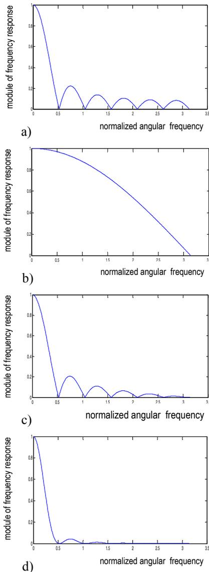
Fig.2 Magnitude frequency responses of the MA filters – a) rectangular impulse response of the length of 12 samples; b) filter with frequency response according to eq.(6); c) filter with frequency response according to eq.(8); d) serial connection of two filters with  $H_1(z)$ .
