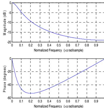
Fig.4 Magnitude and phase frequency response of the filter with exponential weight for smoothing constant a=0.2
