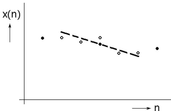
Fig.1 Smoothing of a sequence of five samples by means of a polynomial of the 1<sup>st</sup> order
