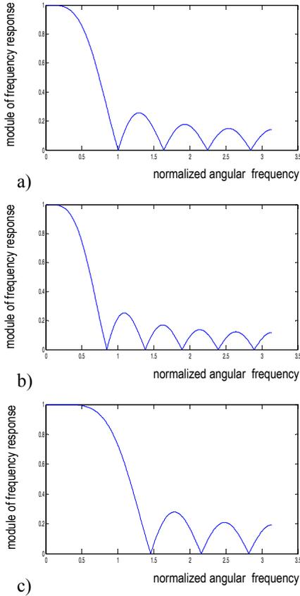
Fig.3 Magnitude frequency responses of filters designed for – a) 3<sup>rd</sup> order polynomial and 11 sample impulse response; b) 3<sup>rd</sup> order polynomial and 13 sample impulse response; c) 5<sup>th</sup> order polynomial and 11 sample impulse response.
