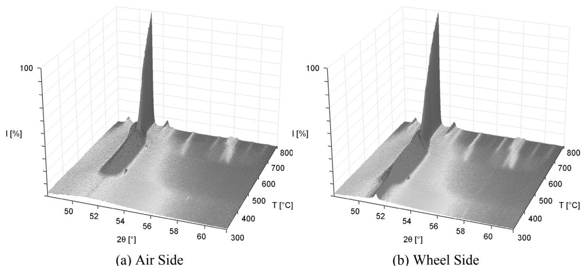
Fig. 1. Diffractograms of the  $\text{Fe}_{79}\text{Mo}_8\text{Cu}_1\text{B}_{12}$  alloy measured *in situ* during linear heating with the rate of  $10^\circ\text{C}/\text{min}$  and arranged into three-dimensional record: (a) the air side of the ribbon, (b) the wheel side of the ribbon.
