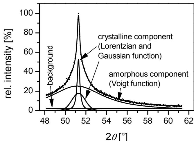
Fig. 2. X-ray diffractogram of the wheel side of the  $\text{Fe}_{79}\text{Mo}_8\text{Cu}_1\text{B}_{12}$  ribbon and its decomposition into corresponding components. It was measured *in situ* at a temperature of  $410^\circ\text{C}$ .
