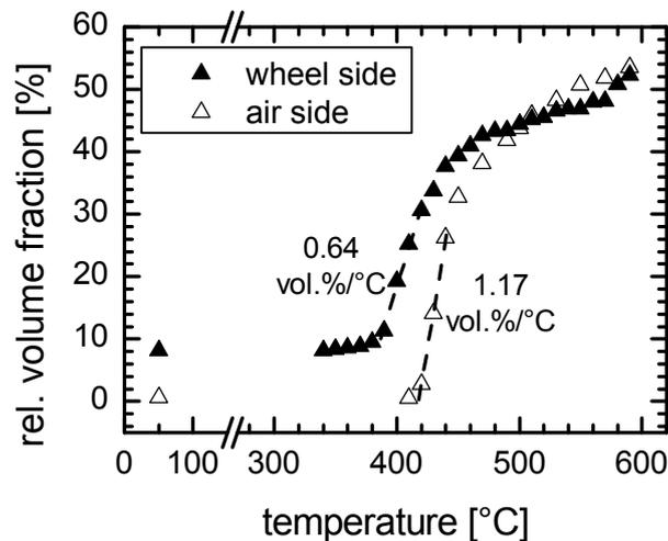
Fig. 3. Temperature evolution of the relative volume fraction of the crystalline *bcc*-Fe(Mo) phase in the Fe<sub>79</sub>Mo<sub>8</sub>Cu<sub>1</sub>B<sub>12</sub> alloy.
