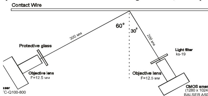
Fig. 2. Optical layout of contact wire wear inspection system.
