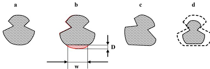
Fig. 1. A contact wire profile and its flaws: an unworn wire (a); a standard defect (b); a “turn” defect (c); “neck” defect (d).
