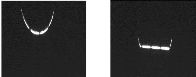
Fig. 3. Real nonprocessed (raw) image of contact wire under structured light for unworn wire (left) and worn wire (right) cases.
