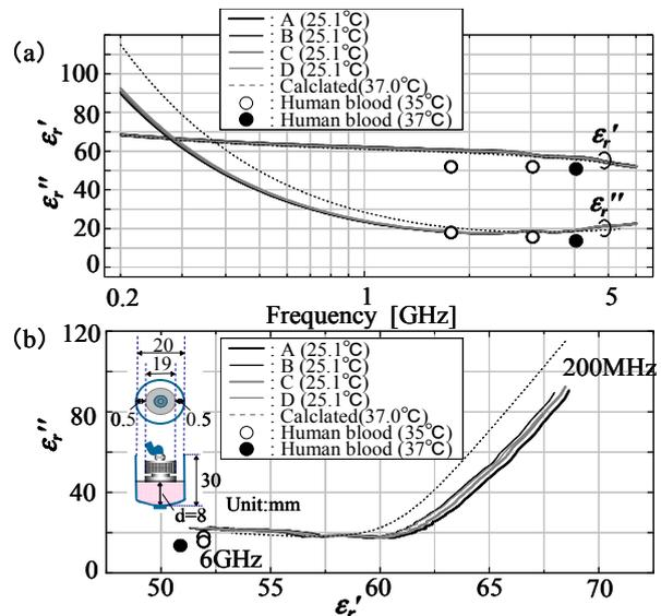
Fig. 4. Measured results of complex relative permittivity of blood for four healthy subjects. (a) frequency characteristics and (b) Cole-Cole plots.
