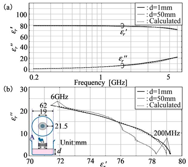
Fig. 2. Measured results of complex relative permittivity when changing distance  $d$  from probe face to bottom of beaker: (a) frequency characteristics and (b) Cole-Cole plots.
