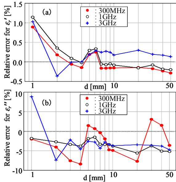
Fig. 3. Relative errors to calculated values of complex relative permittivity when changing distance  $d$  from probe face to bottom of beaker.
