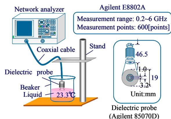
Fig. 1. Measurement setup and open-ended coaxial probe.
