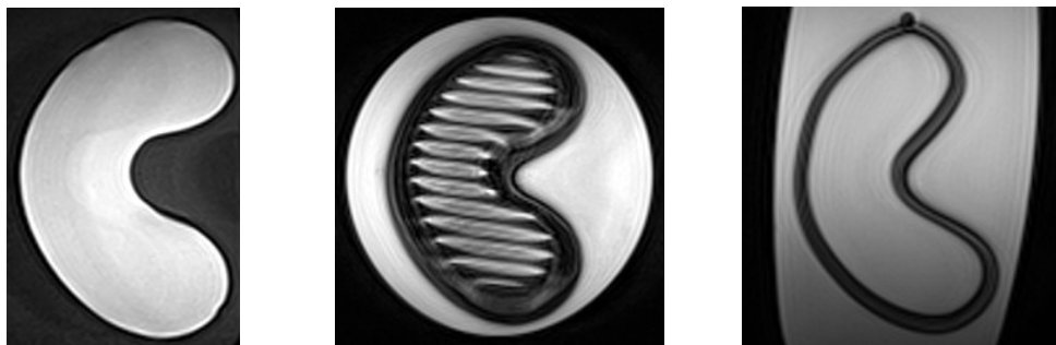
Fig. 3. Left: Image of the oil slick, GRE imaging sequence, TR = 800 ms, TE = 10 ms, slice thickness 2 mm. Center: Image of the soft magnetic sample, GRE, TR = 400 ms, TE = 10 ms, slice thickness 2 mm. Right: Image of the thin coil wire up into the oil slick shape, DC current 20 mA, GRE, TR = 500 ms, TE = 10 ms.
