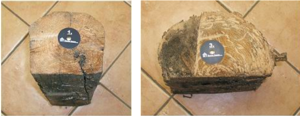
Fig. 2. Examples of wood invaded by decay-fungi and wood-destroying insects.
